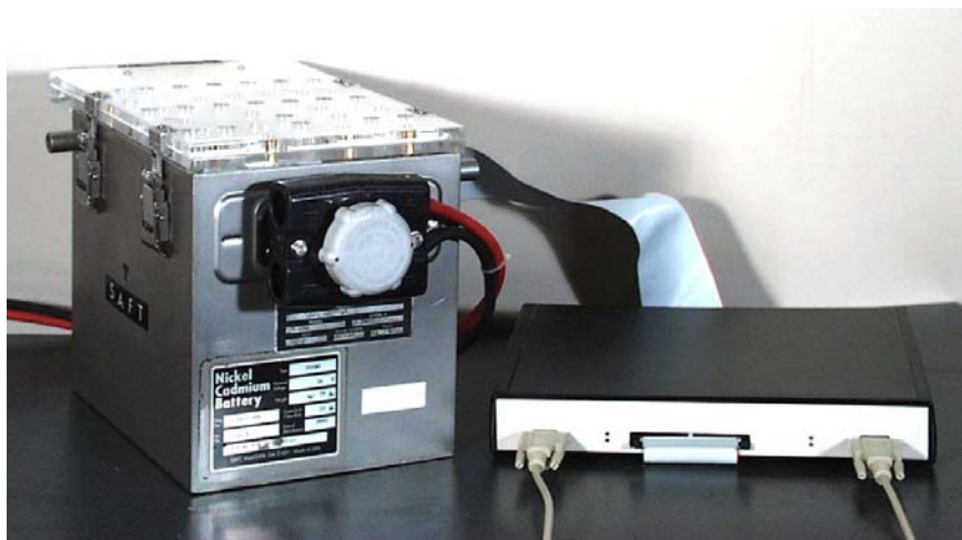
The BTAS16 method of measuring and recording of battery and cell voltage readings. Shown in the picture are the battery specific Crown, which makes contact with the cells and the Data Terminal which takes all the readings and transfers them to the Computer.
