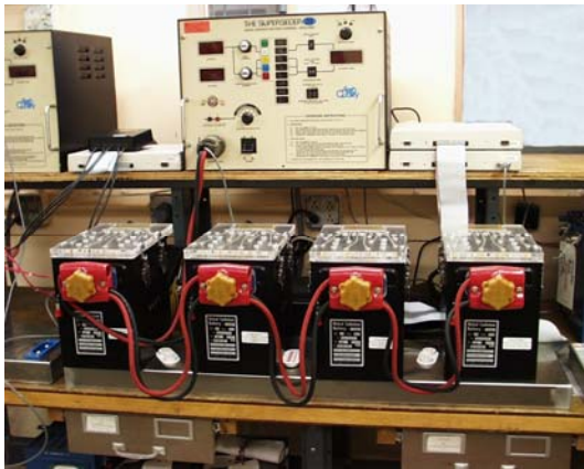
Superseder Charger-Analyzer and two C-Scans provide simultaneous test and analysis of four MD-80 batteries
