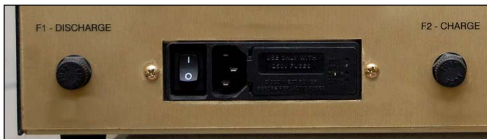
Figure 12 - Power Entry Block and Fuses
