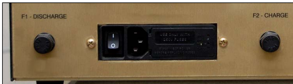
Figure 12 - Power Entry Block and Fuses
