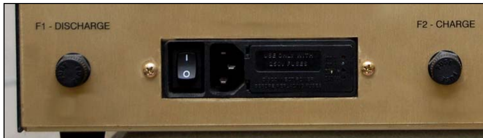
Figure 12 - Power Entry Block and Fuses
