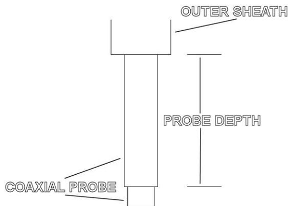
**Figure 2 – Probe Depth**
