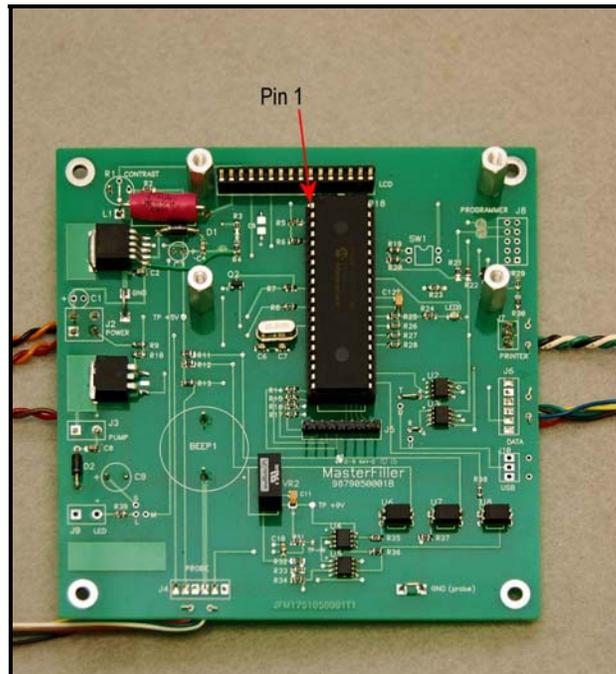
Figure 6 - Installed Processor
