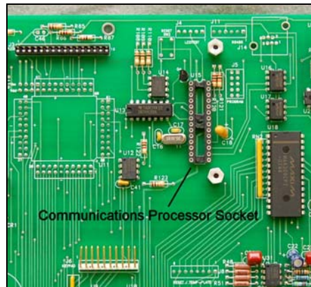
Figure 23 - Communications Processor Socket
