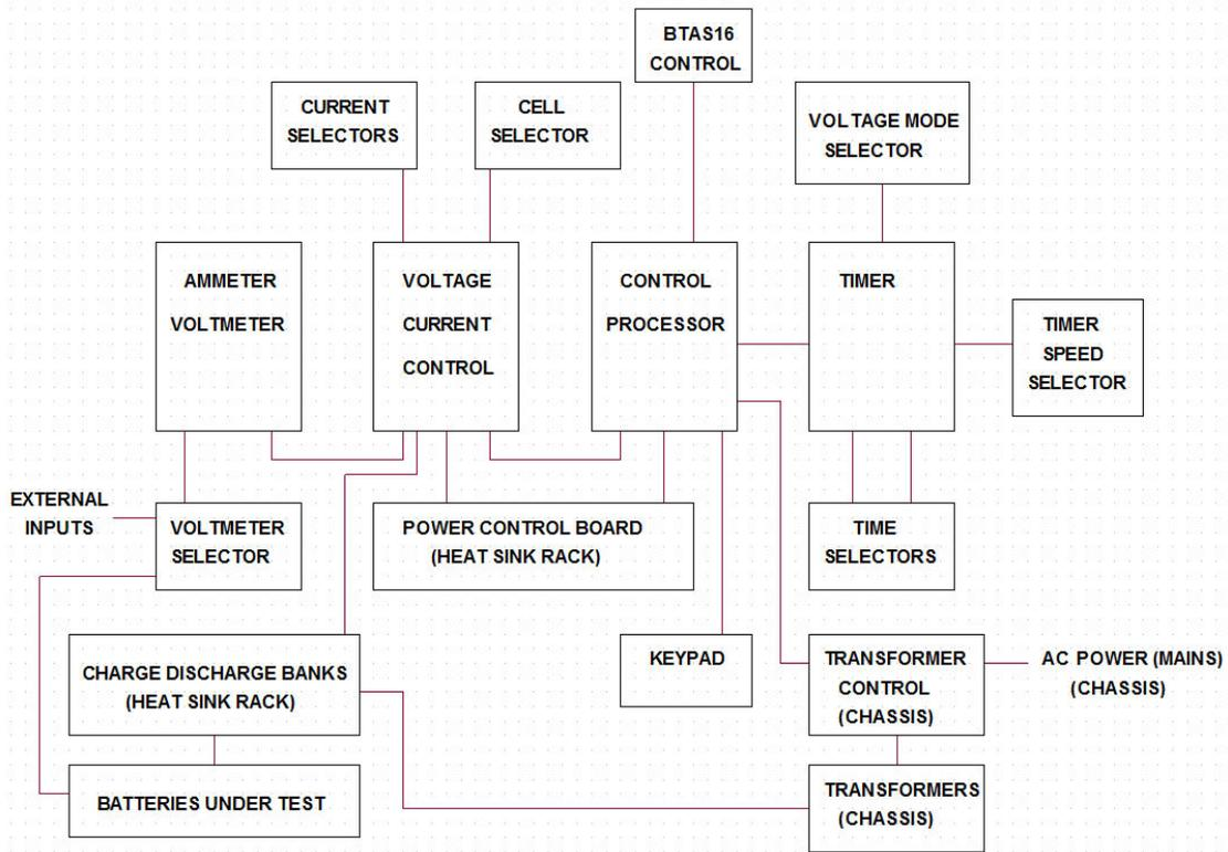
Figure 1 - Block Diagram
