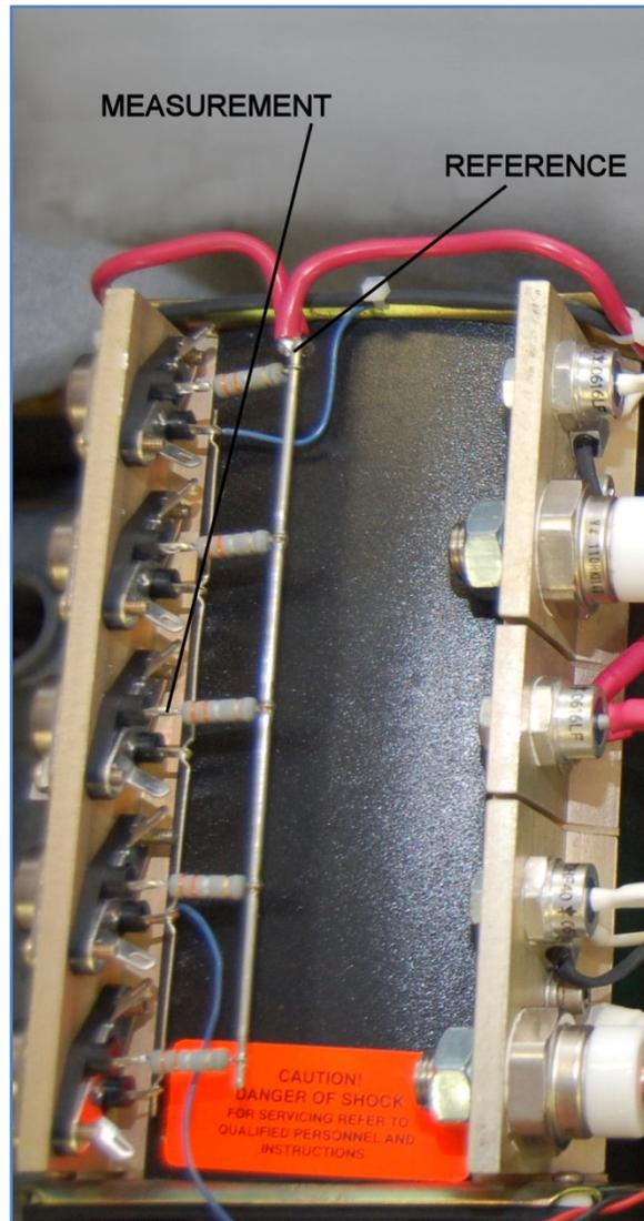
**Figure 9 - Measuring for a shorted transistor**
