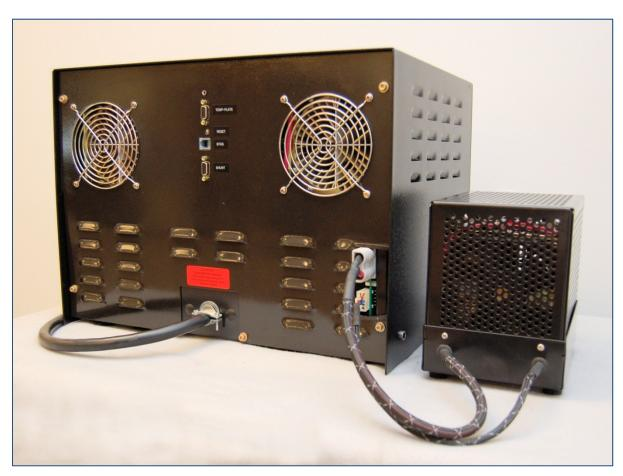
Figure 3 – Connecting the EXD Module to the Charger-Analyzer
